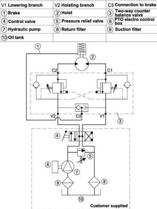
( Powered by PTO / power take off unit driven pump ) The installation of the counterbalance valve supplied is required for 100% braking
