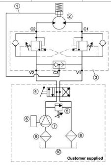
( Powered by PTO / power take off unit driven pump ) The installation of the counterbalance valve supplied is required for 100% braking
